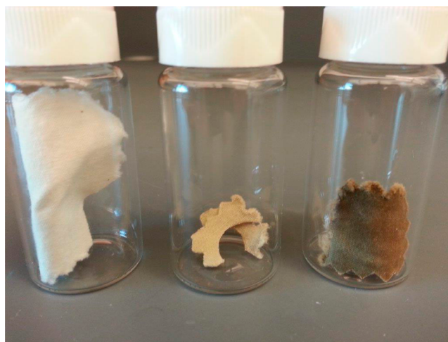
Figure 6. Materials after being exposed to hydrogen sulfide: untreated cotton (left), MOF-cotton (center), and POM-MOF-cotton (right).
